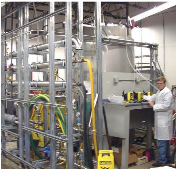
Shaw's 4000-L Fermentor and Cell Concentrator
