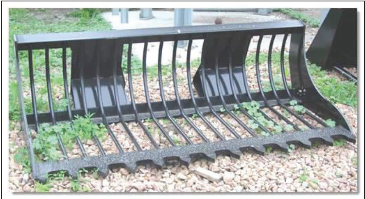
Figure 5. Example of a rock bucket to sort larger artifacts and sort rocks and debris.
